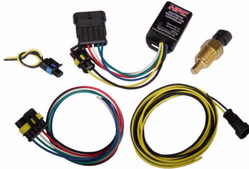
The HPC Radiator Fan Controllers provide control over one or more electric radiator fan(s). The module uses a temperature sensor installed in the engine or radiator to determine when to energize relays to turn on the fan(s). The temperature setting is easily adjustable by rotation of a potentiometer located inside the module. In addition, the module also has a remote override wire which may be connected to an existing air conditioning system or an override toggle switch to turn on the fan(s).
