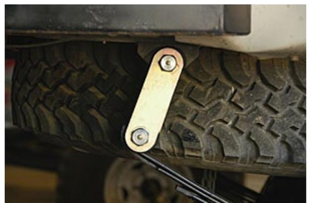
8) Shocks can be installed a number of different ways. They can be mounted so the top of one is tipped forward and the other is tipped backwards. Which is the most common method and is how most Toyota 4x4's came from the factory. For this style of mounting, stock upper shock mounts can be reused.
