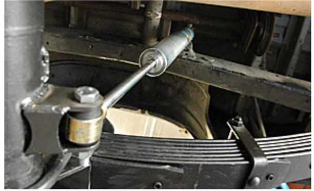
Another method of mounting shocks is to weld a tube between frame rails above the axle and mount the shock from the axle up to the tube. With this method, it will be necessary to angle the tops of the shocks inward to prevent the shock from bottoming out.
