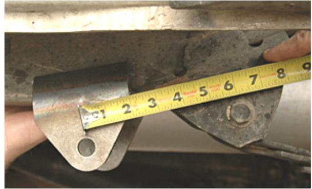
**Note:** Trail-Gear, Inc. rear leaf springs are longer than stock springs and require spring hangers to be relocated further apart.
