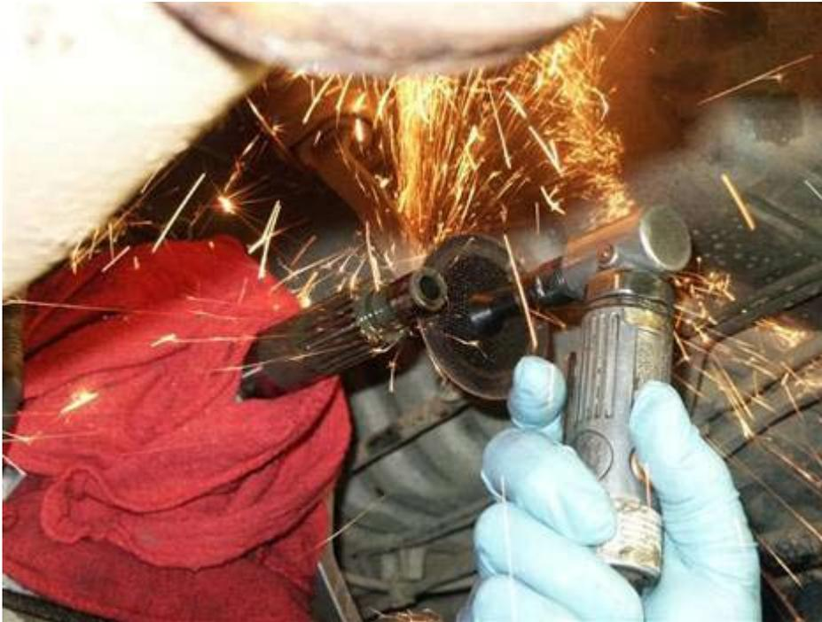
Clean gasket surface and vacuum any remaining shavings from the grinder out of the output shaft.
