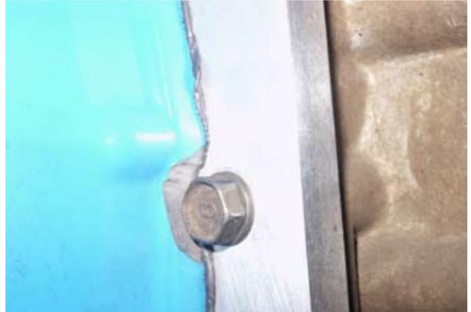
Test fit the adapter, be sure to use bolts with the right thread pitch!
