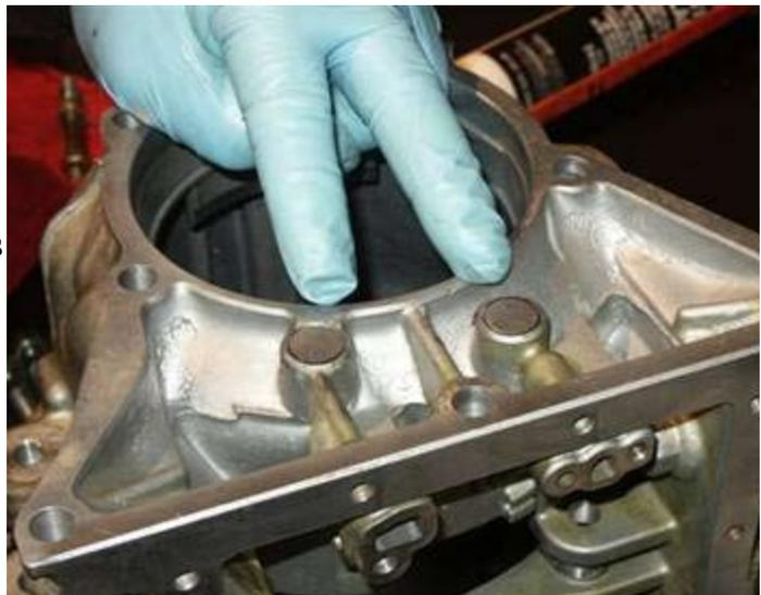
Remove shift shaft oil seal. Install 22mm expansion plug (PN 100-1606) in place of shift shaft oil seal with some gasket sealant.
