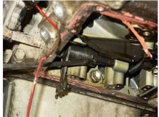
Remove park lock pawl bracket, spring, pin, and pawl. **SAVE** the pin and spring to be reused in the transmission.
