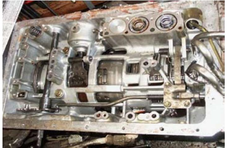
Install valve body. Connect throttle cable. Align groove of manual valve to pin on the shift linkage. Make sure that the springs and check ball are installed correctly.
